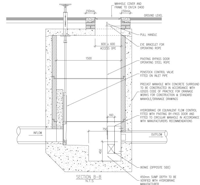
FLOW CONTROL MANHOLE DETAIL
