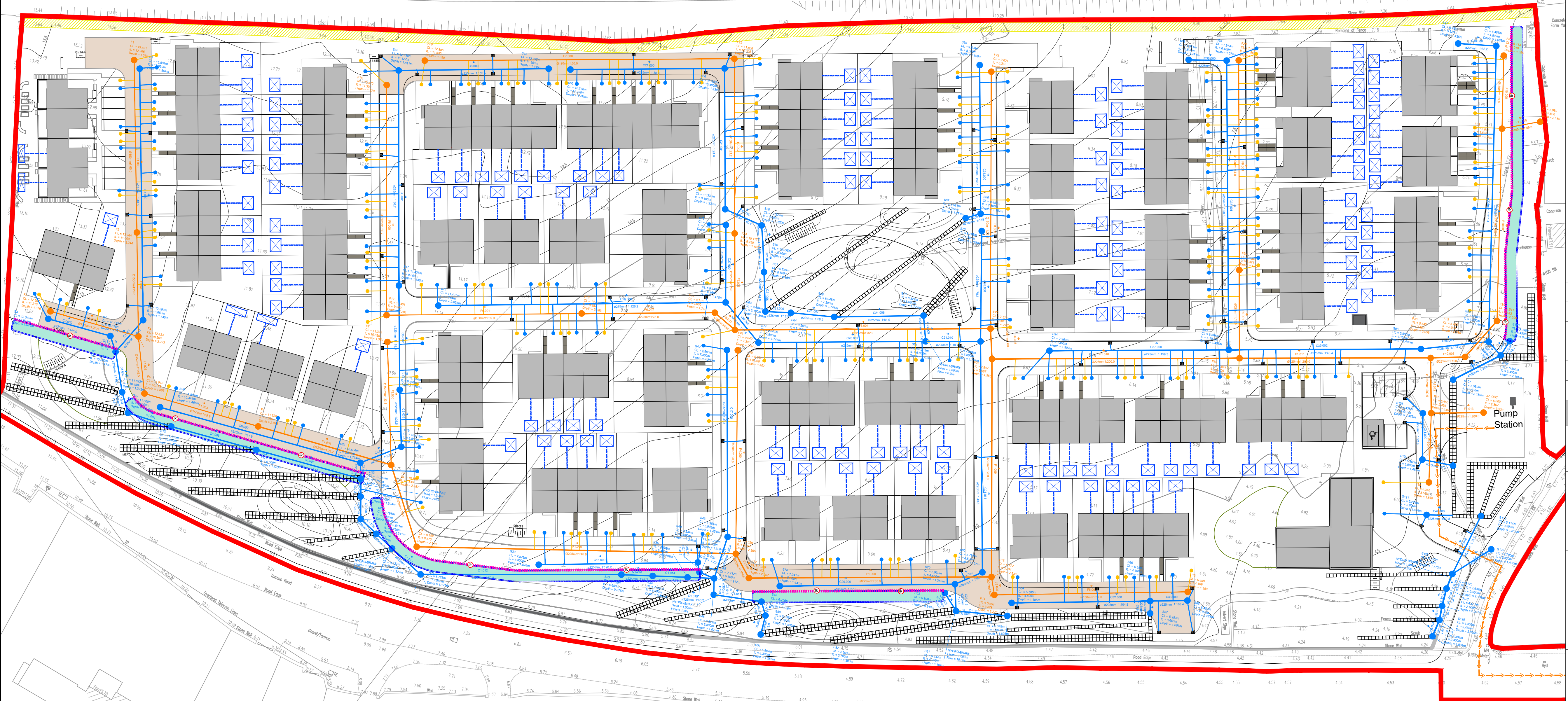
PROPOSED FOUL & STORM WATER LAYOUT SCALE 1:500
