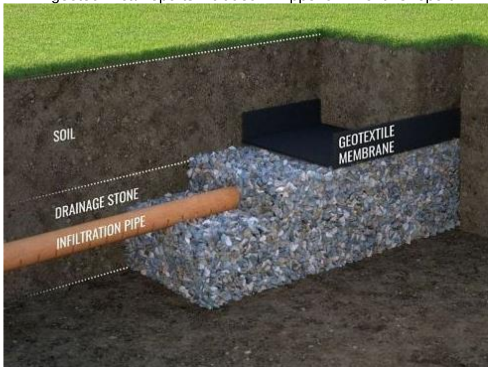
Figure 3.2 Garden Soakaway Example
